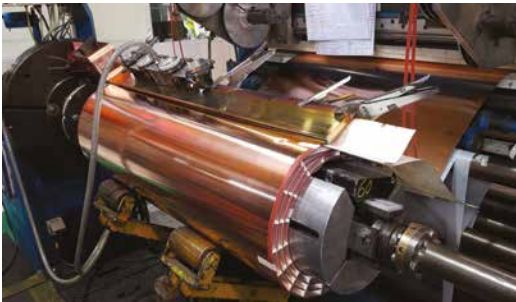
LV winding with foil technology
